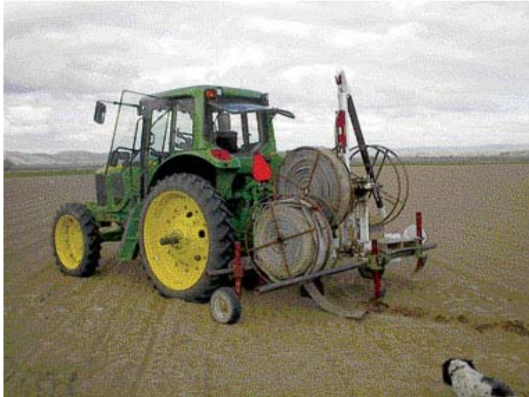
Laying supply hose to drip lines requires manpower, machines and time, but the rest of the season is easy on labor with drip irrigation.
