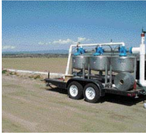
Trailer-mounted portable drip stations are used to pump and filter canal water to drip tape.
