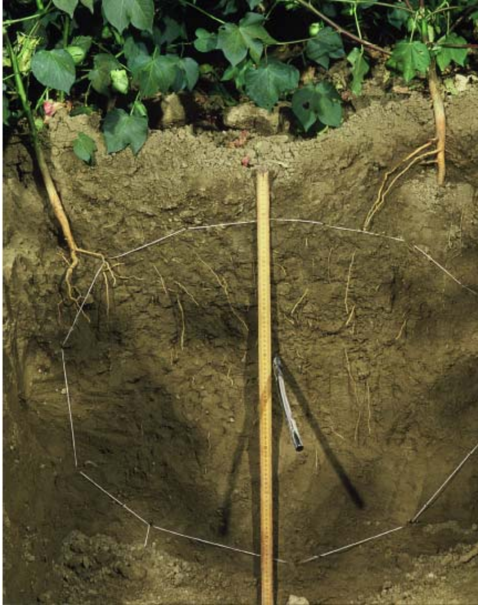
Figure 7a. Wetted patterns created in a dry Panoche clay loam soil using a SDI system with discharge rate of 2 l/h and a high frequency (1-hour) irrigation period.
