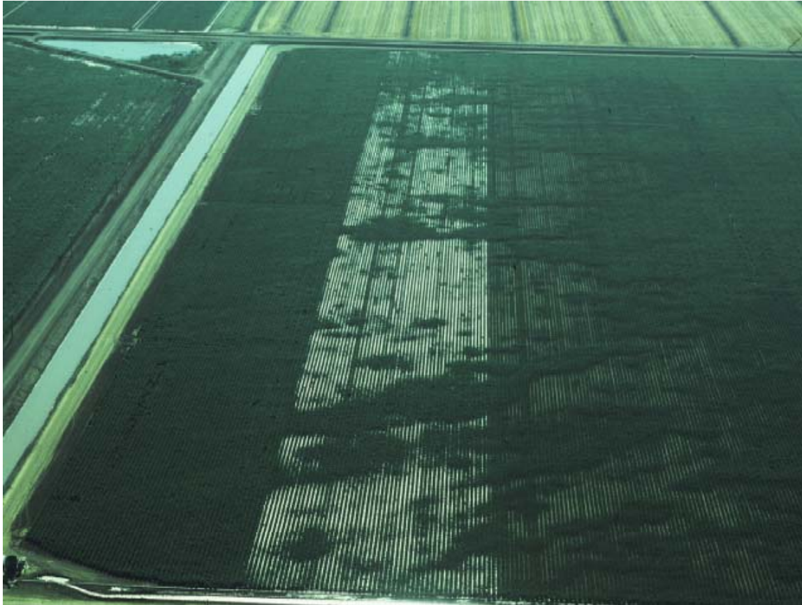
Figure 11. A commercial example of cotton canopy uniformity differences between 10 ac. Irrigated by a SDI system (left hand side), a surge flow irrigation system being irrigated (middle) and a conventional furrow system (right hand side) on July 27, 1987 (Photo courtesy of USDA-ARS, WMRL 1987).
