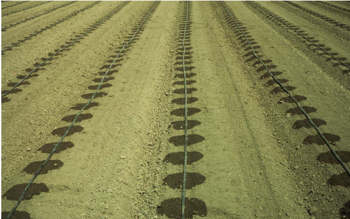
Figure 10. An example of high uniformity soil wetted pattern generated by a two-year old single Drip System (DI) lateral on a 60-in. bed before planting at the UC West Side REC in April 1982.
