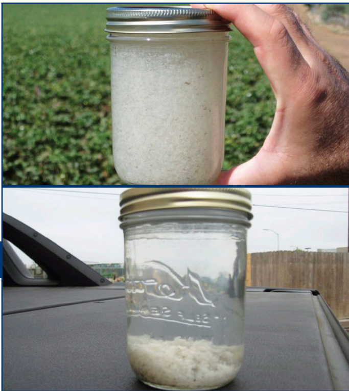
Top: Chemical reaction in jar test of fertilizer and irrigation water forming cloudy precipitate.
